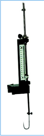
CFRM. Level gauge for measurement of the water height (hook and point gauges)
