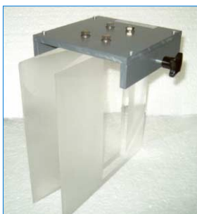
CFVEN. Venturi flume
