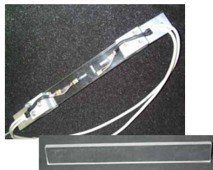
N°10-G. Small Rectangular Specimen with strain gauges + N°10. Small Rectangular Specimen
