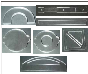
EFO-K4. Kit of Test Specimens with Strain Gauges (advanced kit)
