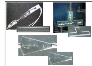
EFO-K3. Kit of Test Specimens with Strain Gauges (basic kit)
