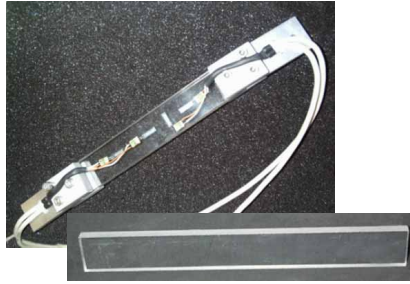
N°8-G. Big Rectangular Specimen with strain gauges + N°8 Big Rectangular Specimen
