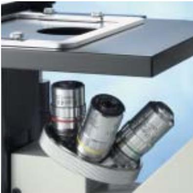
*Nosepiece inverted microscope*
