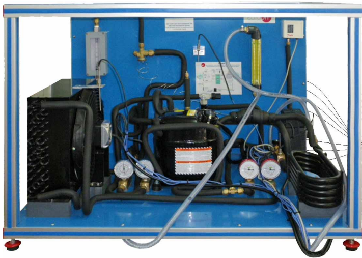
① Unit: THARALC. Refrigeration and Air Conditioning Unit (one condenser (air) and one evaporator (water))
