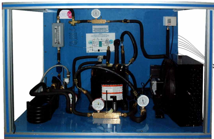
① Unit: THALAC. Air Conditioning Unit (one condenser (water) and one evaporator (air))
