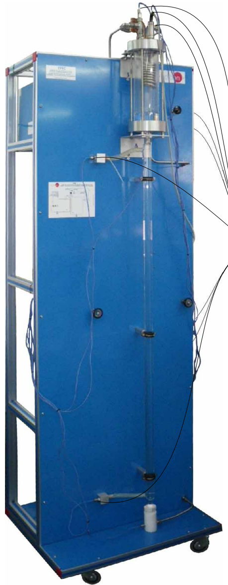
① Unit: TFEC. Flow Boiling Demonstration Unit
