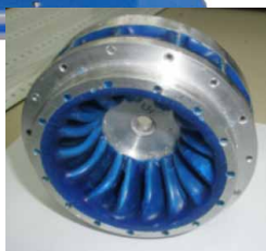
Detail of the turbine
