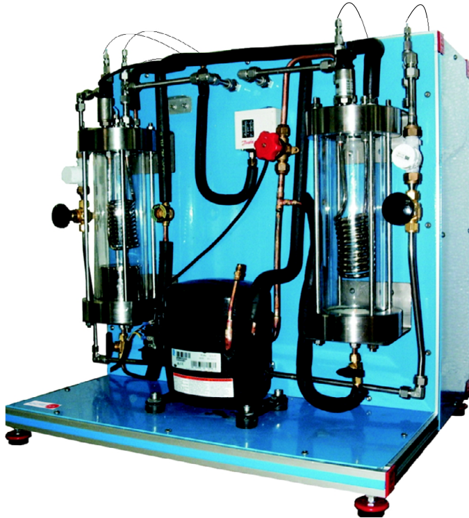
① Unit: TCRC. Refrigeration Cycle Demonstration Unit
