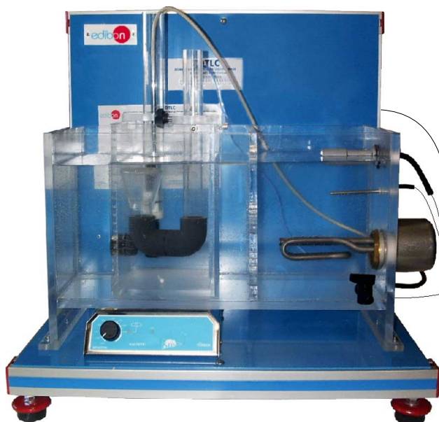
① Unit: QDTLC. Liquid Mass Transfer and Diffusion Coefficient Unit
