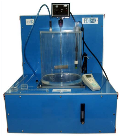
① Unit: PEAIC. Aeration Unit
