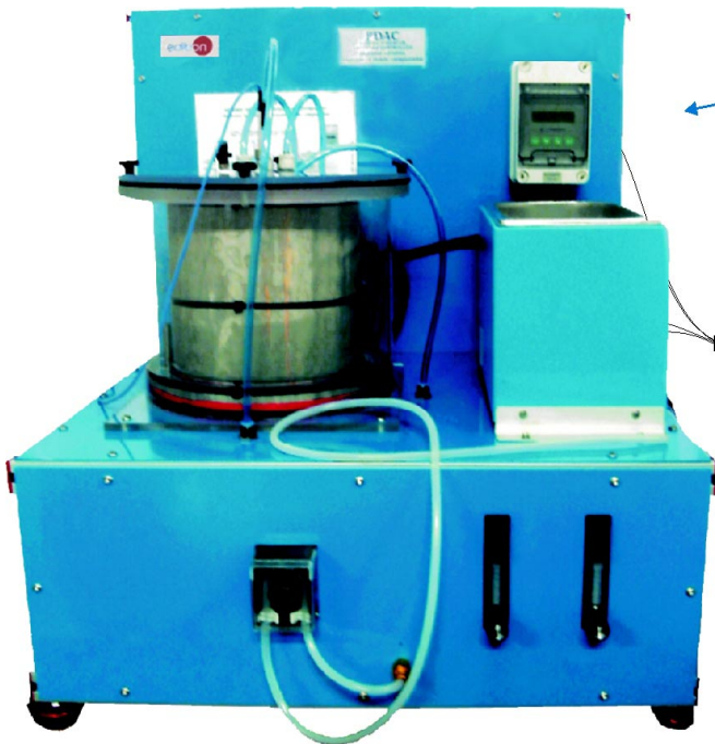
① Unit: PDAC. Aerobic Digester
