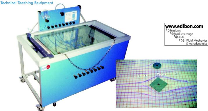
The Laminar Flow Visualization and Analysis Unit allows a complete study of the two-dimensional problems associated with the laminar flow by means of the visualization of the different models of flow that can be visualized with the help of an efficient system of injection of coloured liquid. It is an amplification of the Hele-Shaw apparatus.
