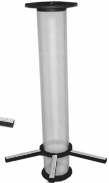
HVCB-CTPG. 144mm. duct and pressure taking with Pitot
