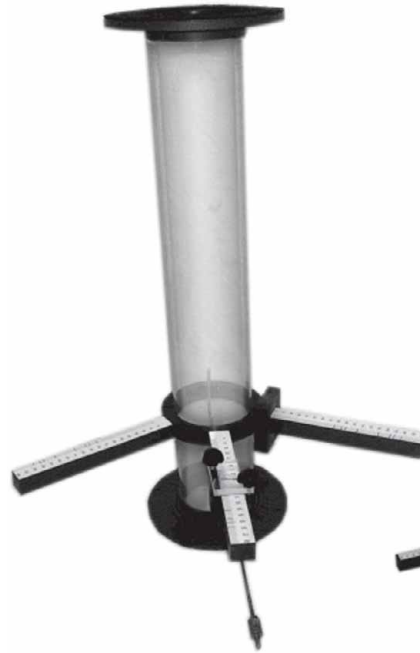
HVCB-CTPP. 94mm. duct and pressure taking with Pitot
