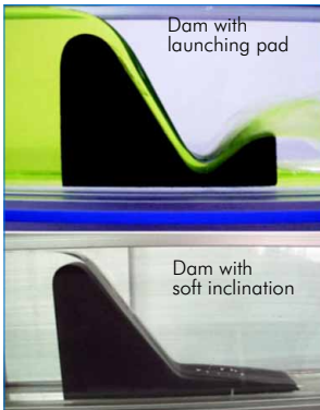
CFGCPVP. Dams spillway and flow splitters (3 different models of dams)
