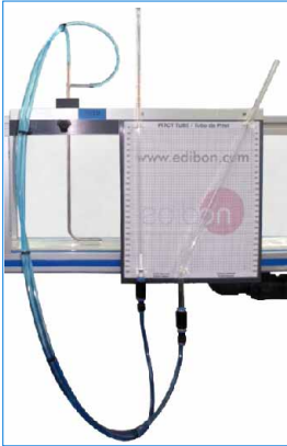
CFGCTP. Pitot tube and manometer board
