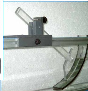
CFGCCVR. Vertical flat gate and radial gate
