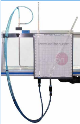
CFTPC. Pitot tube and manometer board
