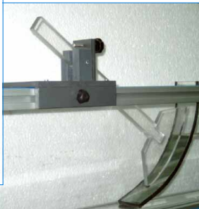
CFCVRC. Vertical flat gate and radial gate
