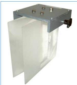
CFVEN. Venturi flume
