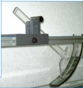
CFCVR. Vertical flat gate and radial gate
