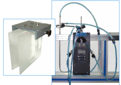
CFTVC. Venturi tube, with pressure transducers, converter and differential pressure digital indicator for input flow measurement
