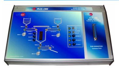
It represents a liquids blending control where is possible to emulate the mix of different liquids and their flows are regulated using four valves.
