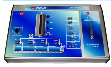
It represents a pump control where we have four pumps inserting water in a big tank.
