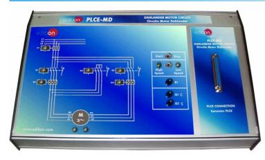
It represents a Dahlander motor which has two connections of velocity with 2 and 4 poles and emulates the motor's movement.
