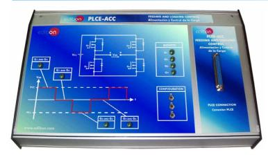
It represents a feeding and loading control system where we can control the voltage in the load between the A-B terminals.
