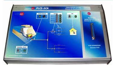
It represents a channeling system where we have a dam which provides water using a general pipe with a general valve.
