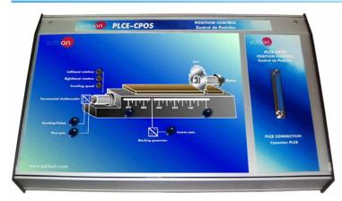
It represents a position control where we can move the sheet to the correct position using a motor with a lefthand and righthand rotation and crowling speed the incremental shaft encoder can count pulses and to give a fine sincronism.
