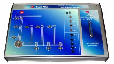
It represents a motor with two separate windings and emulates the motor's movement.
