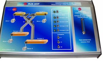
It represents a conveyor charging system where is possible to emulate the work of four conveyor belts switching on/off their motors and we can open or close three lock gates.
