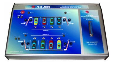
It represents a car parking where is possible to emulate the elements used in a typical car parking like barriers, vehicles presence detectors, traffic lights, fire sensors.
