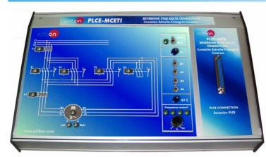
It represents a reversing motor with star-delta connection in the secondary and emulates the motor's movement.
