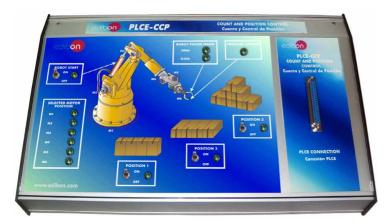
It represents a count and position control where is possible to emulate the robot's movement selecting the general final position. It shows with lights the final selected position of each motor. We can know when the robot is opening or closing its hand and when it has taken a piece with light signals.
