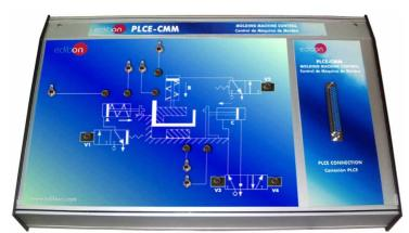
It represents a molding machine control where we can emulate a machine which gives shape to the pieces pushing them.
