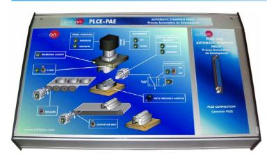
It represents an automatic stamping press where is possible to emulate the pressing process of steel sheets.
