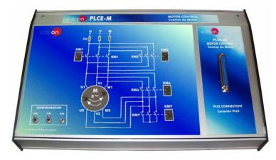
It represents a motor control where is possible to emulate the movements of a three-phase motor with both turning directions controlled by three-phase contactors.
