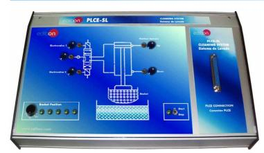
It represents a cleaning system where is possible to emulate the movement of a basket which has vertical movements.
