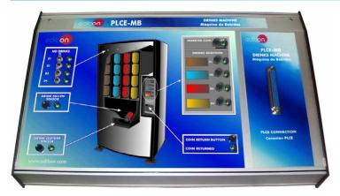
It represents an automatic drinks machine where we have the possibility of work with a complete scheme of actions of an automatic drinks machine.
