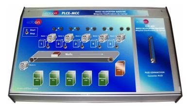
It represents a collecting belt conveyor system where is possible to emulate five conveyor belts transporting different materials to the general conveyor belt.
