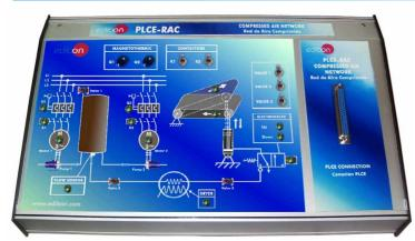
It represents a compressed air network where is possible to emulate the actions in an air network.
