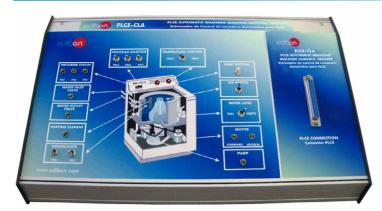
It represents an automatic washing machine control allowing to emulate the sequence of actions carried out by a washing machine.
