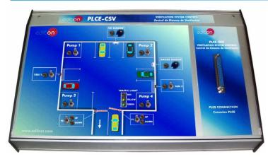
It represents a ventilation system control where we are trying to clean the air in a garage.
