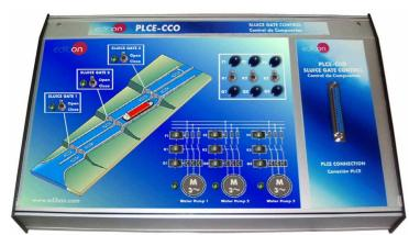
It represents a sluice gate control where we can see three sluice gates and we have to control them using the water pumps and the gates control.
