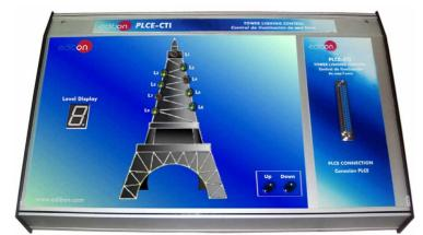
It represents a tower lighting control where is possible to emulate the lighting of different levels of a tower using a lights system.
