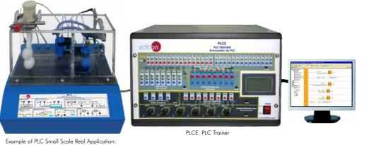
PLCE-BS6. Liquid Level Test Module
