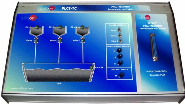
It represents a coal treatment system where we can see three chutes with three valves each one and a big tank. We can control the flow of coal with the three valves and is possible to know if the tank or the chutes are full using coal presence sensors.
