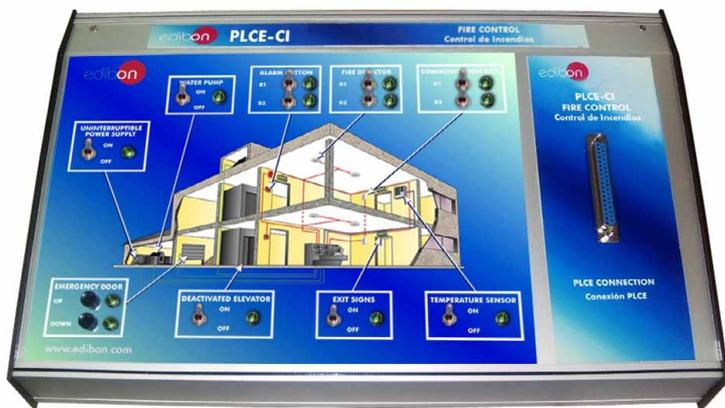
It represents a fire control station where is possible to emulate different emergency situations with fire.
