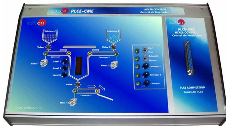
It represents a mixer control where we can emulate the mix with two different products in a big chute from two little chutes using conveyor belts, finally the general conveyor belt will transport the mix. We will control the motors of the conveyor belts and the valves in the system and we will know the big chute's level using sensors.
