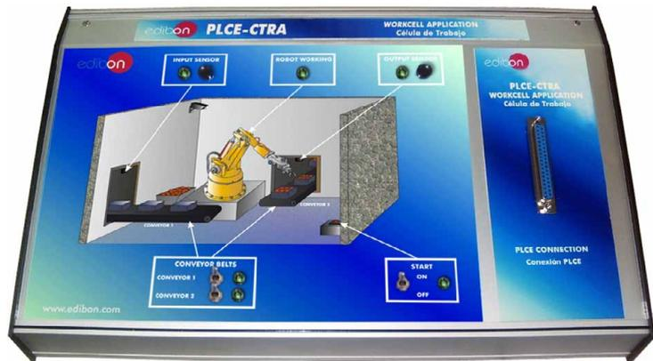
It represents a workcell with a robot inside where is possible to emulate the automatic work of a robot and the conveyor belts. We can activate or deactivate the conveyor belts and start/stop the general system. We have input and output sensors and a light which indicates when the robot is working.
