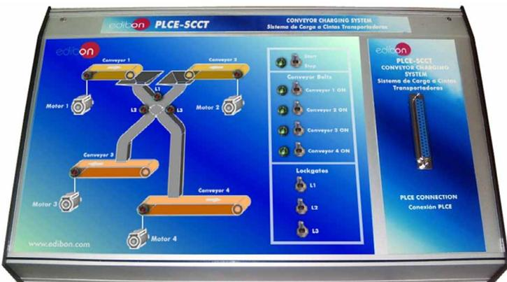
It represents a conveyor charging system where is possible to emulate the work of four conveyor belts switching on/off their motors and we can open or close three lock gates.
