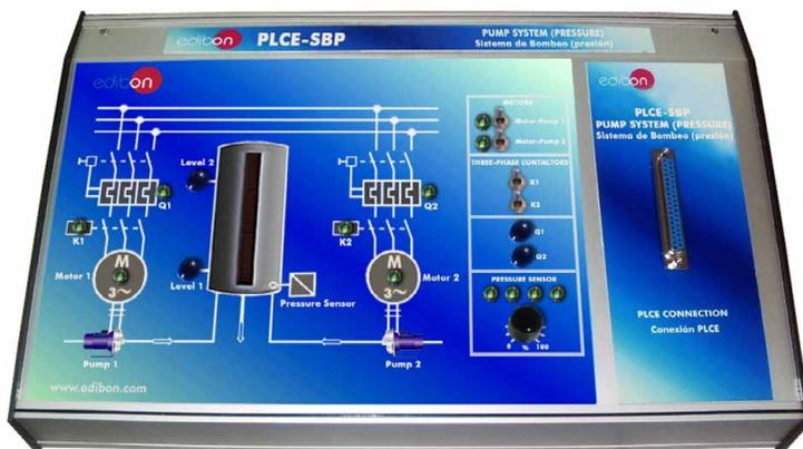
It represents a pressure system where we use two pumps with their motors when we have to introduce air in the tank.
