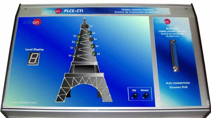
It represents a tower lighting control where is possible to emulate the lighting of different levels of a tower using a lights system. It has two directions up and down and we can know the level using a display.
