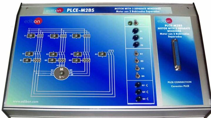
It represents a motor with two separate windings and emulates the motor's movement. Is possible to switch on/off the motor and to connect the different windings and the secondary with the three-phase contactors. We can simulate faults with the three-phase fuses and the magnetothermics.
