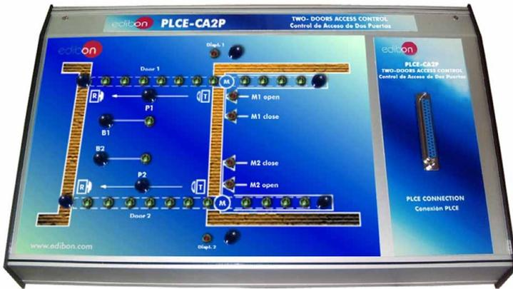
It represents two automatic doors where is possible to emulate the movements and positions of each automatic door using sensors and electrical motors.
