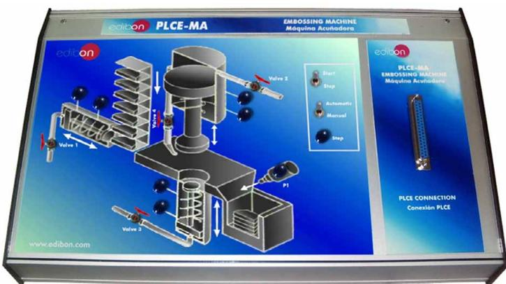
It represents the embossing process of metal disks controlled with an electropneumatic system.
