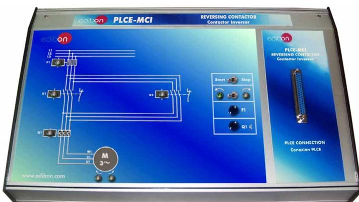
It represents a three-phase motor with reversing contactors and emulates the motor's movement.
