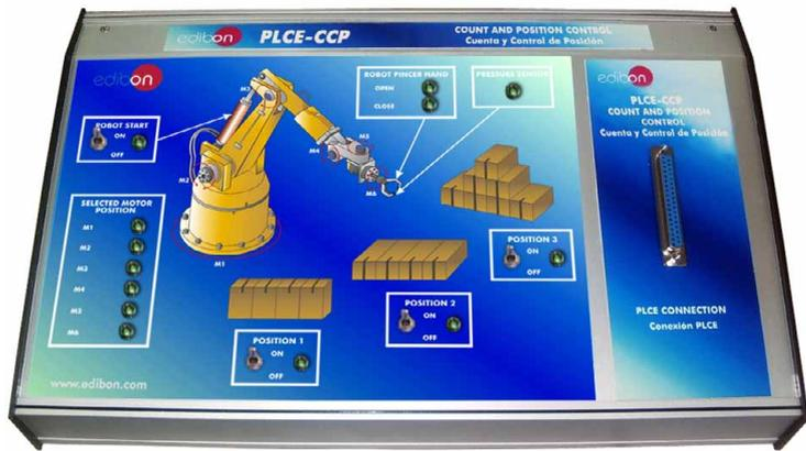
It represents a count and position control where is possible to emulate the robot's movement selecting the general final position. It shows with lights the final selected position of each motor. We can know when the robot is opening or closing its hand and when it has taken a piece with light signals.
