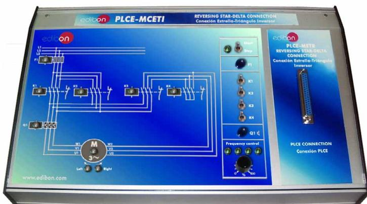
It represents a reversing motor with star-delta connection in the secondary and emulates the motor's movement.
