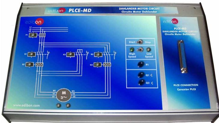
It represents a Dahlander motor which has two connections of velocity with 2 and 4 poles and emulates the motor's movement. Is possible to switch on/off the motor in both turning directions and to connect it with 2 or 4 poles using the three-phase contactors. We can simulate faults with the three-phase fuses and the magnetothermics.
