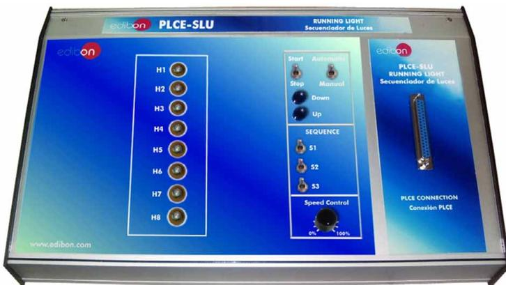
It represents a running lights system where we can emulate the control of the eight lights in different speed, sequence and direction.
