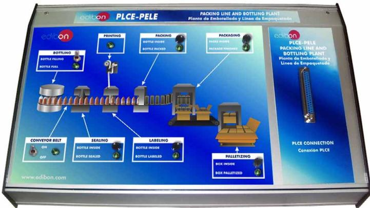
It represents an automatic packing line and bottling machine where is possible to emulate the processes of bottling, sealing, labeling, packing and palletizing. In this automatic plant we can control the movement of the conveyor belt and to obtain information about the process using sensors.
