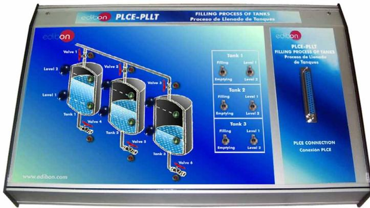
It represents a filling process of tanks with three tanks where we can emulate the filling and emptying processes of the tanks and the level of the liquid inside the tanks.
