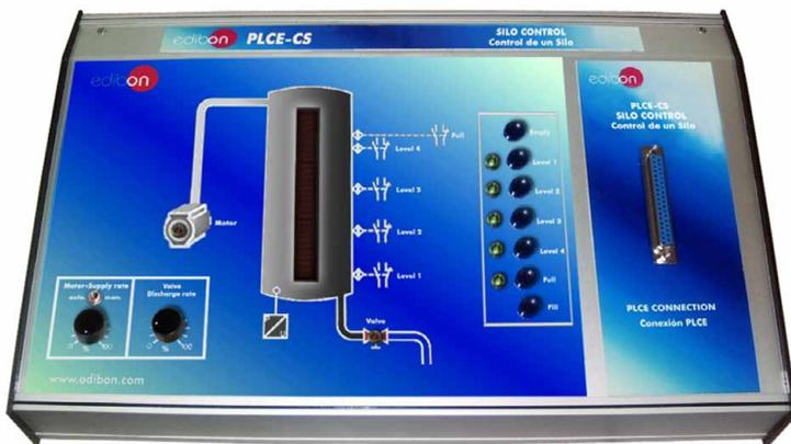
It represents a silo control system where we can emulate the filling process. The filling motor has a manual rate or an automatic rate and the output valve has its own discharge rate. We can measure the level with four presence sensors and to know if the silo is full with the full sensor.
