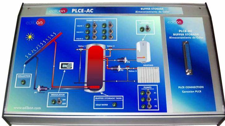
It represents a buffer storage system where is possible to emulate the storage of heat using fluids.
