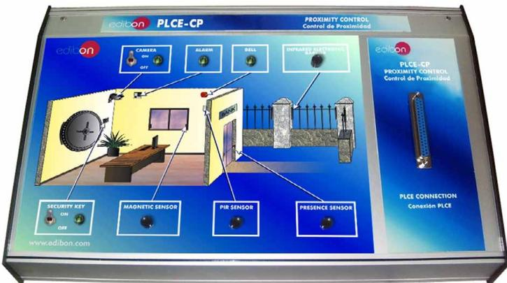
It represents a proximity and presence security control where we can obtain information about the presence in different places of a bank office using a PIR sensor, presence sensor, magnetic sensor and infrared electronic barriers.
