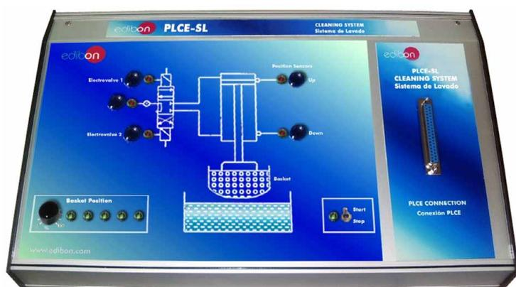
It represents a cleaning system where is possible to emulate the movement of a basket which has vertical movements.
