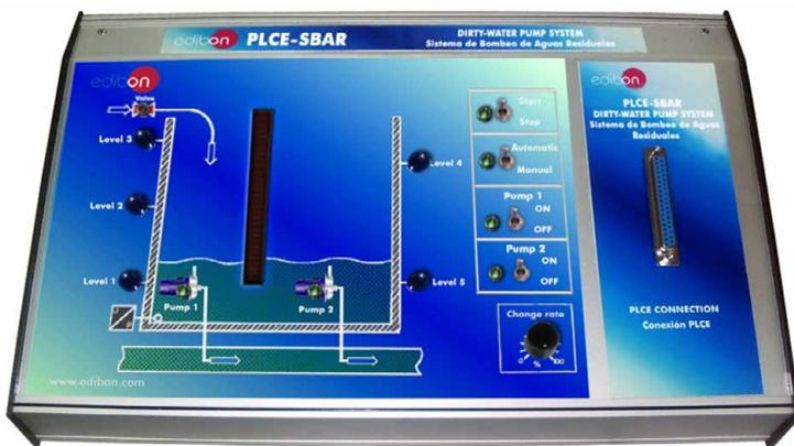
It represents a dirty-water pump system where we can emulate the control of the dirty-water flow using a valve and two pumps which insert dirty-water in the pipe from the dirty-water tank.
