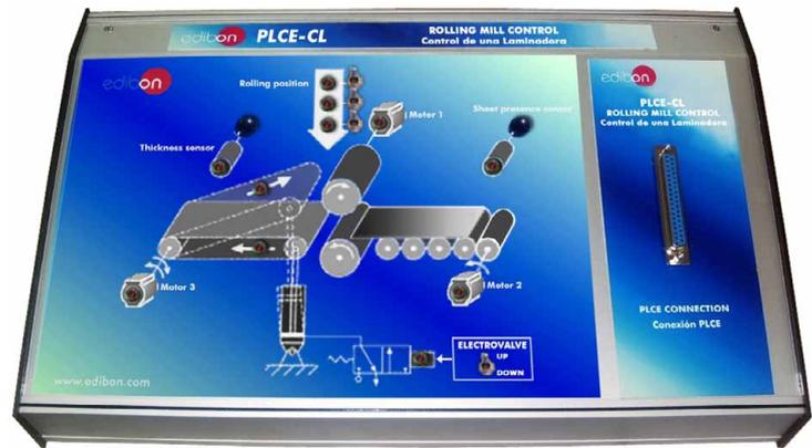
It represents a rolling mill control where is possible to emulate the position of rolling mill, the movement of the different motors and the position of the conveyor belt using an electrovalve. We can obtain information about the presence and the thickness of each sheet of metal using sensors.
