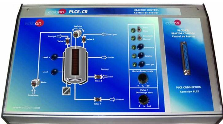
It represents a reactor control where is possible to emulate the mix of a catalyst, an inert gas and the substance. We can regulate the catalyst and the inert gas flow with valves, and the substance with a pump. The inlet and the output of the product are regulated using valves. We mix the substances with an agitator into the reactor.
