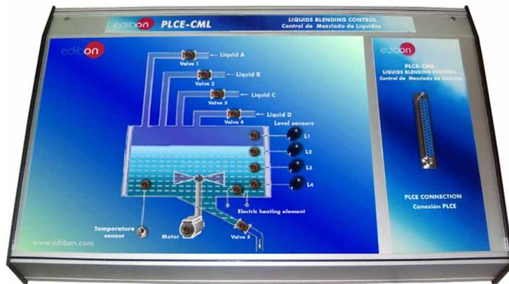
It represents a liquids blending control where is possible to emulate the mix of different liquids and their flows are regulated using four valves. The liquids are mixed using a mixer with its own motor. The flow of the mix is regulated using an output valve. We can measure the temperature and the level of liquid with sensors.
