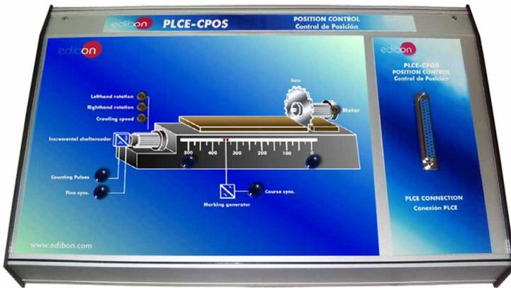
It represents a position control where we can move the sheet to the correct position using a motor with a lefthand and righthand rotation and crawling speed the incremental shaft encoder can count pulses and to give a fine sincronism. We have the possibility of saw the sheet connecting the saw motor.
