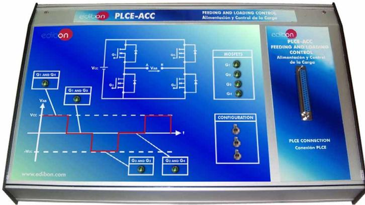
It represents a feeding and loading control system where we can control the voltage in the load between the A-B terminals. We have to select a configuration which activate or deactivate the mosfets and we can know what switch is closed with its own light. We can see in the graph the state of the voltage in the load between the A-B terminals.
