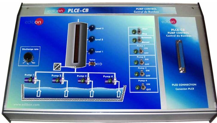
It represents a pump control where we have four pumps inserting water in a big tank.
