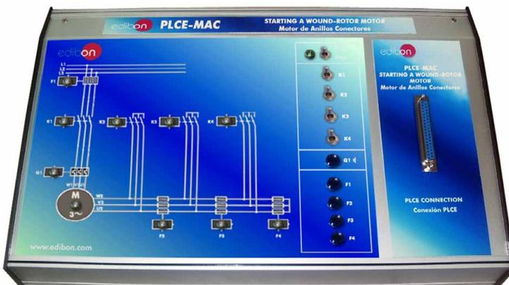
It represents the starting of a wound-rotor motor where is possible to emulate the motor's movement. Is possible to switch on/off the motor and to connect the secondary with different loads with the three-phase contactors. We can simulate faults with the three-phase fuses and the magnetothermics.
