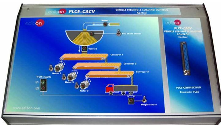
It represents a vehicle feeding control where we use three conveyor belts to transport the material to the vehicles. We can switch on/off each conveyor belt and the valves. We have two traffic lights which can indicate when the vehicle can start its movement and a weight vehicle sensor.
