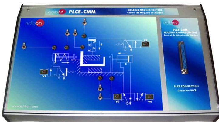
It represents a molding machine control where we can emulate a machine which gives shape to the pieces pushing them.
