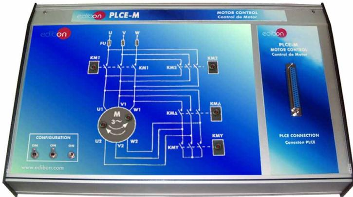
It represents a motor control where is possible to emulate the movements of a three-phase motor with both turning directions controlled by three-phase contactors.
