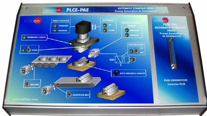
It represents an automatic stamping press where is possible to emulate the pressing process of steel sheets.
