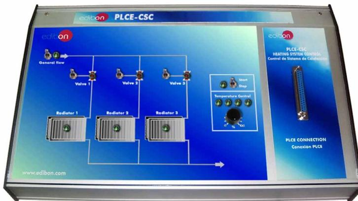
It represents a heating system control where is possible to emulate the heating process controlling the flow of hot water into the circuit activating or deactivating the valves in the pipes and using the temperature control regulator.
