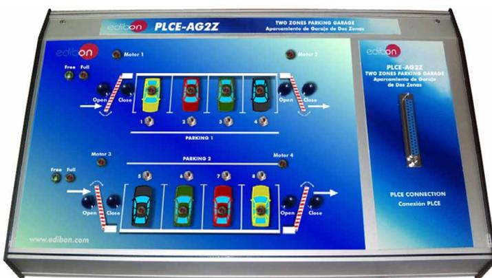
It represents a parking garage with two zones where is possible to emulate the control of four barriers, two in the entrances and two in the exits, in the automatic parking.
