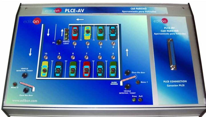
It represents a car parking where is possible to emulate the elements used in a typical car parking like barriers, vehicles presence detectors, traffic lights, fire sensors.
