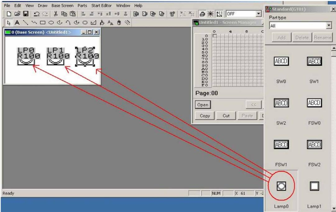
The Touch Screen programming software tool allows to easily create custom screens for PLCE programs. Also some elements can be included by dragging and dropping from libraries.
