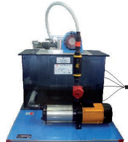
① Unit: TPC. Pelton Turbine
