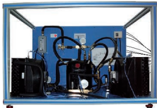
① Unit: THAAAC. Air Conditioning Unit (one condenser (air) and one evaporator (air))
