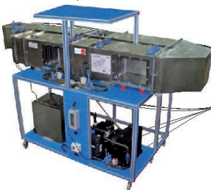
① Unit: TARC. Recirculating Air Conditioning Unit
