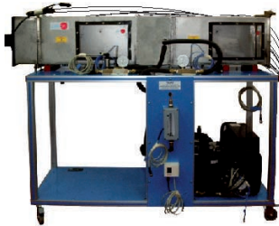
① Unit: TAAC. Air Conditioning Laboratory Unit
