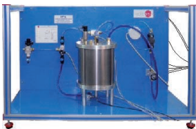
① Unit: TFTC. Nozzle Performance Test Unit
