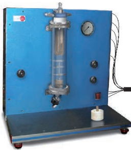
① Unit: TIVAC. Steam to Water Heat Exchanger
