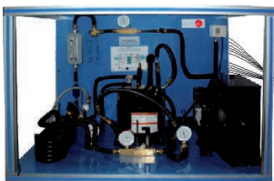
① Unit: THALAC. Air Conditioning Unit (one condenser (water) and one evaporator (air))
