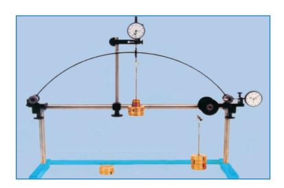
The apparatus enables the student to determine experimentally the horizontal component of the abutment thrust of a simple two hinged arch beam.
