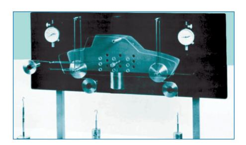
Under conditions of braking or acceleration of a road vehicle, a load transfer between front and rear wheels occurs. The problem of load transfer arises since the accelerating or braking force is not applied to the centre of gravity of the vehicle but to the point of contact of the wheels with the road.
