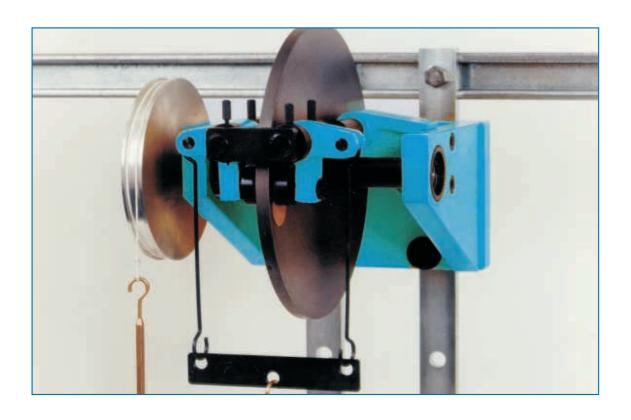
Disc Brake Apparatus has been designed specifically for Motor Vehicle Courses and may be used effectively for classroom demonstrations. It may also be used by the student in the laboratory to carry out simple experiments to investigate the relationship between the normal force acting on the brake pads, the effective radius of the brake pads and the braking torque.
