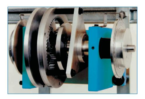
Overdrive Unit has been designed to demonstrate the action of the gear elements in simple epicyclic gear arrangements. The unit may also be used by students in the laboratory to carry out simple experiments on epicyclic gearing.
