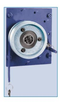
Belt Friction Apparatus has been designed to allow students to carry out investigations to compare the driving torque for a given degree of overlap of
