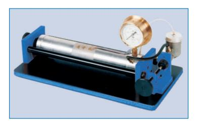
Thin Cylinder Apparatus permits the investigation of stresses and strains in a thin cylinder under internal pressure.
