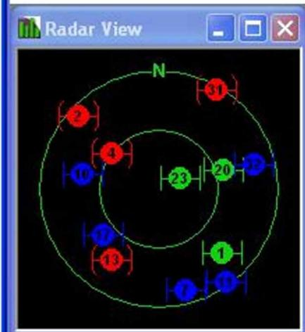
Geographic Azimuth for the positioning of the satellites on the geographic plane together with its identifier, the Azimuth value and the altitude.
